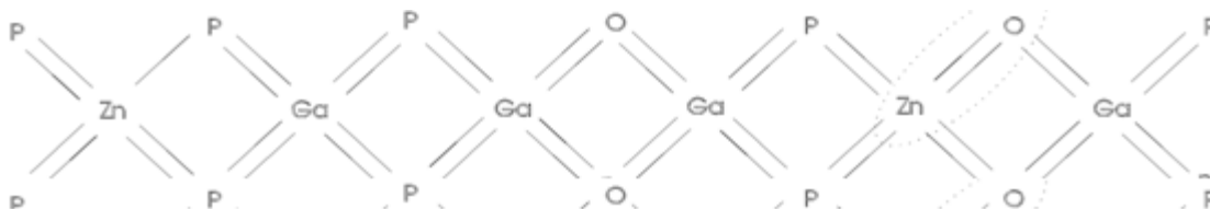
Fig. 10 Doping of GaP with Zn-O.
