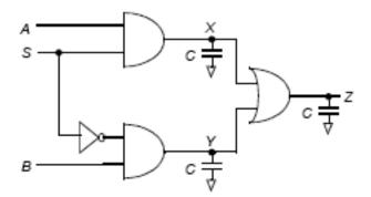
Compute the switching power consumed by the multiplexer shown above assuming that all significant capacitances have been lumped into the three shown capacitors where C=0.3pF. Assume that  $V_{\rm DD}$ =2.5V and the inputs A,S, and B are independent and uniformly distributed with events occuring at a frequency of 100MHz.
