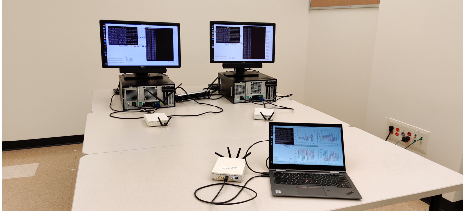
Figure 1.14: GR-WiFi MU-MIMO testbed with 1 AP (laptop) and two STAs (desktops) where real channel response is shown at the AP side.
